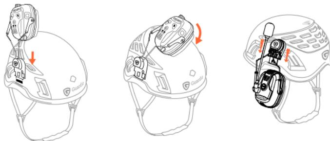
Press the adapter wires inwards to the head until the headset is tightly fitted around the ears. Make sure to adjust the position of the earcup so that it completely cover your earsto avoid any noise leakage.
